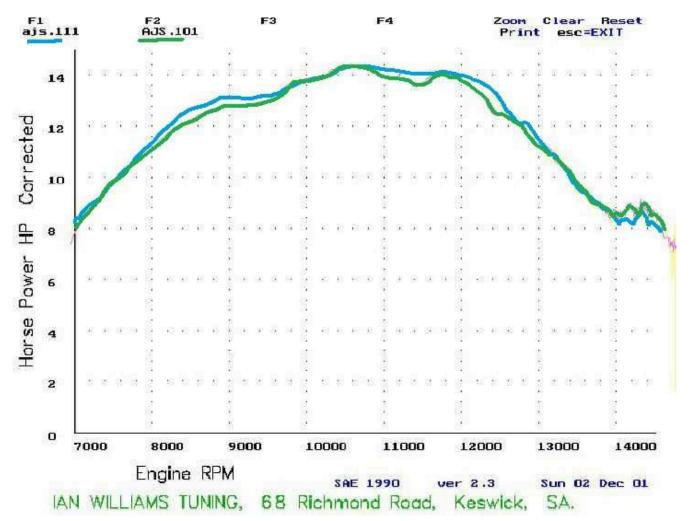
Below are curves for a blueprinted KT100S as #Grunt041 (green line) 'before' and #Grunt044 (blue line) 'after' treatment.
