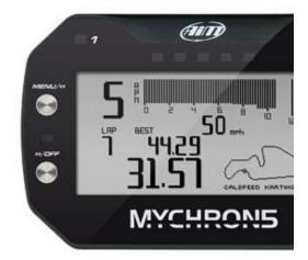
In case your kart is a shift kart, you can decide to show the gear number, automatically calculated in a few hundredths of meters while you are driving.
