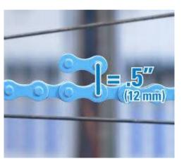
Chain tension needs to be equal to the up and down of 2 widths of your chain. With clutches fitted to almost all karts now, the chain cannot be pulled so tight that it causes the clutch drum to be tilted one way which is what happens if there is not enough slack in the chain.
